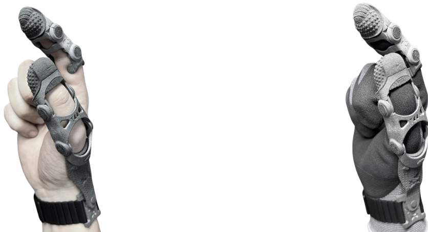
Figure 1. Thumb and index configuration of the ARTUS exoskeleton. Right: With assembly gloves. Left: Without gloves [Not recommended]
